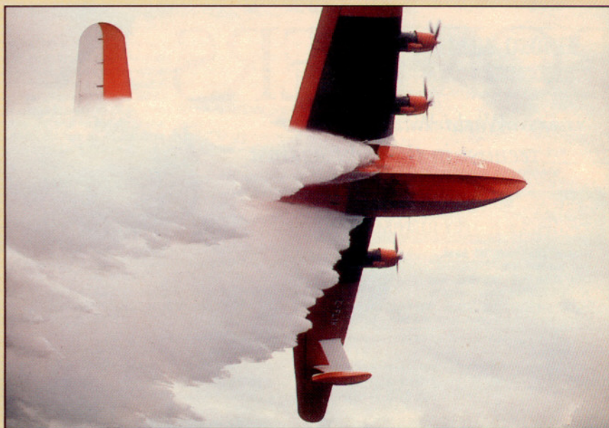
This 1945 photograph (above) shows a Navy Mars taxiing home to the Patuxent NAS. Push a button and 7,200 gallons hit the fire (right); 50 feet agl gives best water impact.
